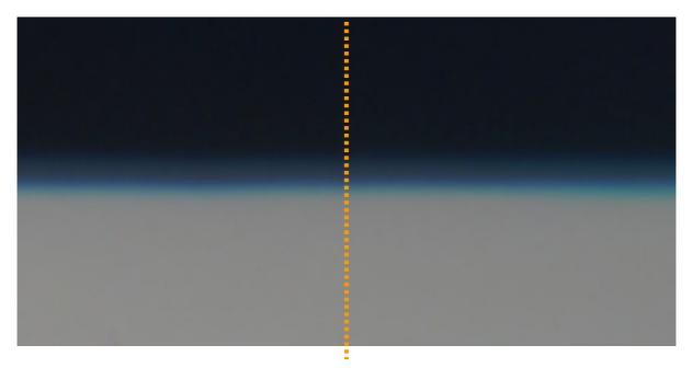
For selected positions along the x-axis of the rectified limb, loop along a line perpendicular to the x-axis in steps of constant length, and for each of the three color channels, calculate the difference of
