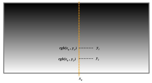
This corresponds to a numerically determined partial derivative of the square-root encoded brightness values with respect to the axis perpendicular to the limb.
