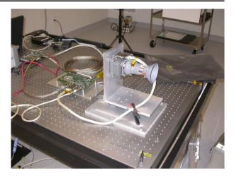
mapped back to focal plane position using a camera model. Analysis of the dot positions shows that the spin axis is within 2 milliradians of the CCD column axis, well under the maximum requirement of 7.8 milliradians imposed by one column of crosstrack drift in 128 TDI steps.
