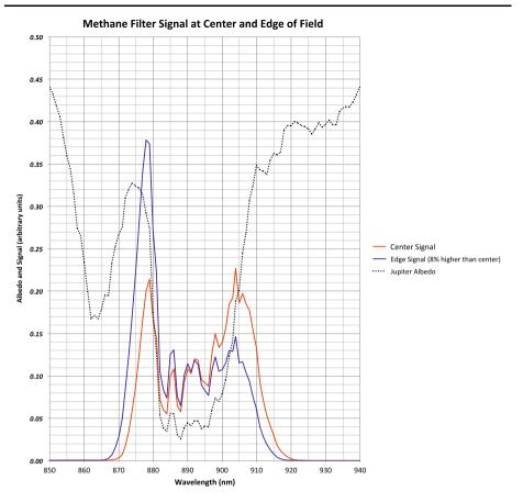
**Fig. 14** Bandpasses are shown for Junocam's methane filter with expected relative signal from the center (*red*) vs. the edges (*blue*) of the field, as described in the text. The *dotted line* shows Jupiter's albedo (Karkoschka 1994)
