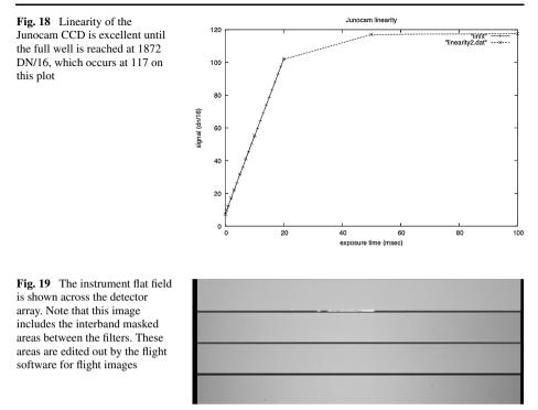
constructed and a stretched version is shown in Fig. 19. (Exposure times used were 0.5 ms for red, 1 ms for green, 5 ms for blue, and 10 ms for methane.)
