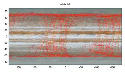
**Fig. 30** Junocam footprints are outlined in *red* for the first 8 orbits. The *green lines* show the spacecraft nadir track for one orbit. The coverage from a single spacecraft rotation forms a "bowtie" on the planet with its narrowest part at the nadir and its widest at the visible limbs; the total size of the bowtie increases with increasing spacecraft altitude. On this simple cylindrical projection, the complete coverage of the poles is not shown
