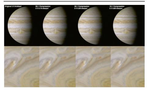
Fig. 28 Different levels (labeled) of simulated image compression are shown. As radiation damage accumulates the commanded level of compression will be adjusted
