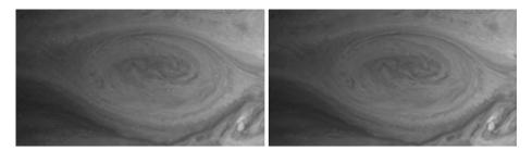
**Fig. 16** Simulated Junocam visible image showing transient effect of high particle flux, for the worst case point in the orbit (perijove +0.4 h). The left image shows simulated hot pixels from radiation. The right image is the left image after median filtering (which is done by Junocam before compression).
