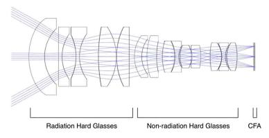
Fig. 15 The raytrace for the Junocam optics is shown
