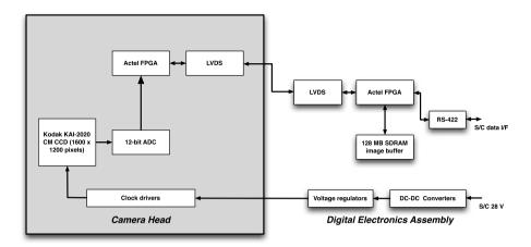
Fig. 11 Junocam electronics functional block diagram
