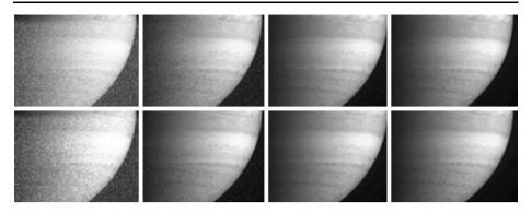
**Fig. 17** Simulated Junocam methane-band image showing transient effect of high particle flux, for points in the orbit (left to right: perijove +0.4 h, perijove +0.5 h, perijove +0.63 h and perijove -0.32 h). The *upper set of images* shown is without median filtering, the lower set is with median filtering. The median filter removes the transient artifacts for the -0.32 h and +0.63 h cases, but not for the +0.4 and +0.5 h cases
